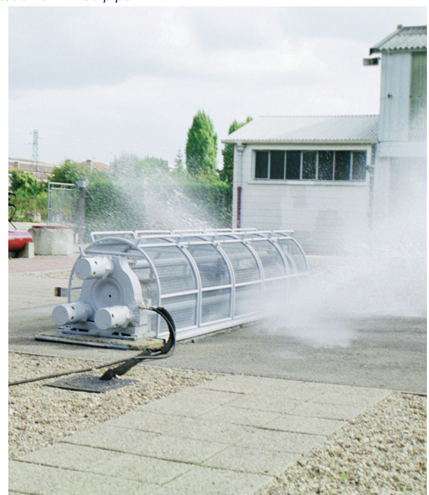
Destructive pressure test on a DN 250 pipe
