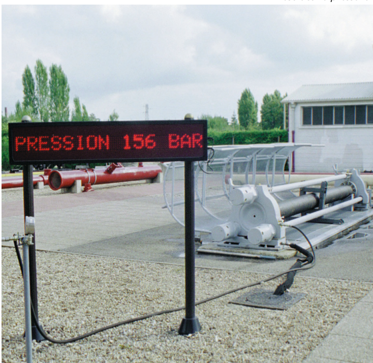
Destructive pressure test on a DN 250 pipe
